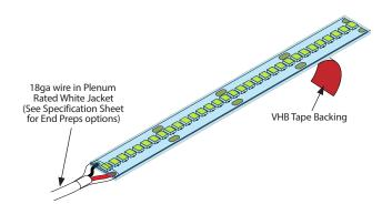
**Caution:** Do not bend, twist or crimp the lead wire at the solder connection point. This will damage the product and void the warranty.
